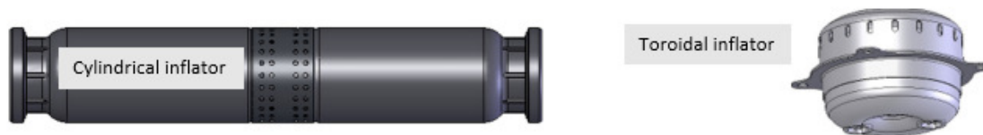
Figure 1. Comparison of a cylindrical inflator vs. a toroidal inflator
